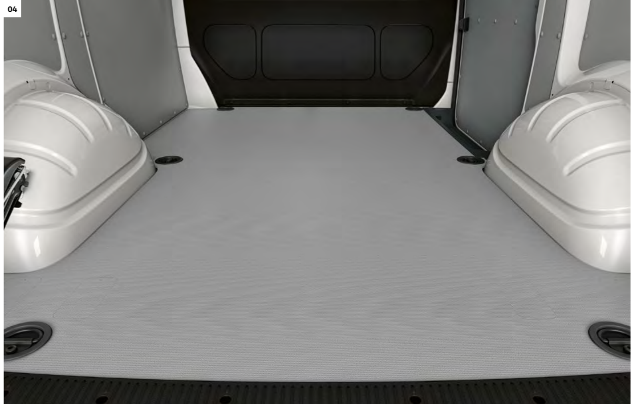
04 Universal floor (for fittings). The ideal preparation for subsequent installation of cabinet systems from various manufacturers 3 . Special adapters 4 in the recesses in the floor covering permit flexible installation of cabinet systems at any time without gluing or drilling. Subsequent removal of the floor leaves only minimum traces. Optional on panel van models. |S|H|
