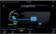
The energy flow display informs the driver about the battery's charge level and the energy flow between the electric motor and high-voltage battery.
