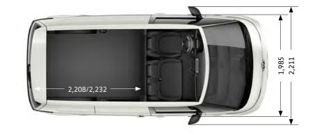
Please note: Vehicle drawings are not to scale. All dimensions in millimetres (mm), unless otherwise stated. The height measurements listed may vary by ± 40mm depending on model and equipment fitted.
