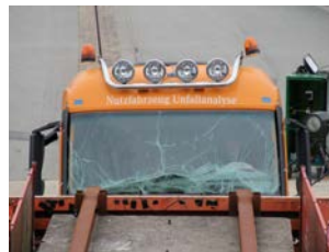
Bending and breaking test: Roof lamp brackets in the crash test.
