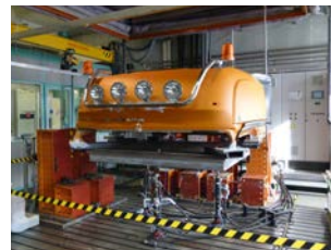
Hydropulse test stand for simulating pot holes and rough road conditions.
