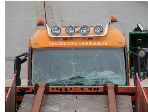
Bending and breaking test: Roof lamp brackets in the crash test.
