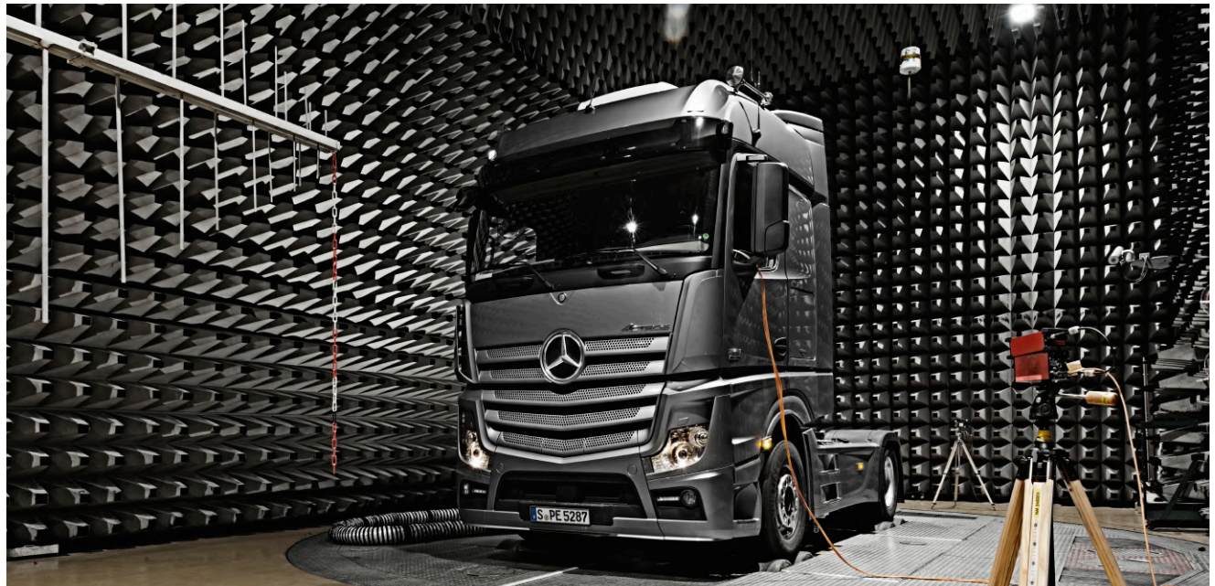
EMC test in a laboratory that is especially shielded against external electromagnetic interferences.
